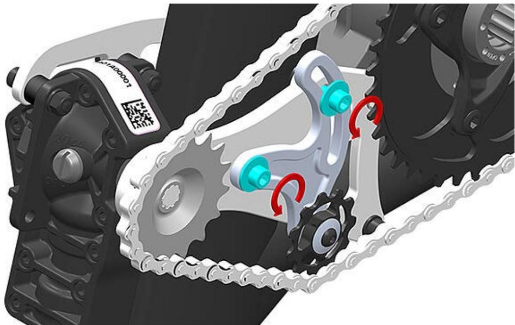
**INFORMATION:** For the purpose of removing the Chain, only loosen the screws by one or two turns sufficient to release Chain tension.
