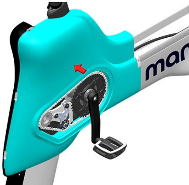
6.3 Fit all seven Buoyancy Clips to secure both LH and RH Buoyancy halves to the hydrofoiler. [Tools: Long Nose Pliers]
