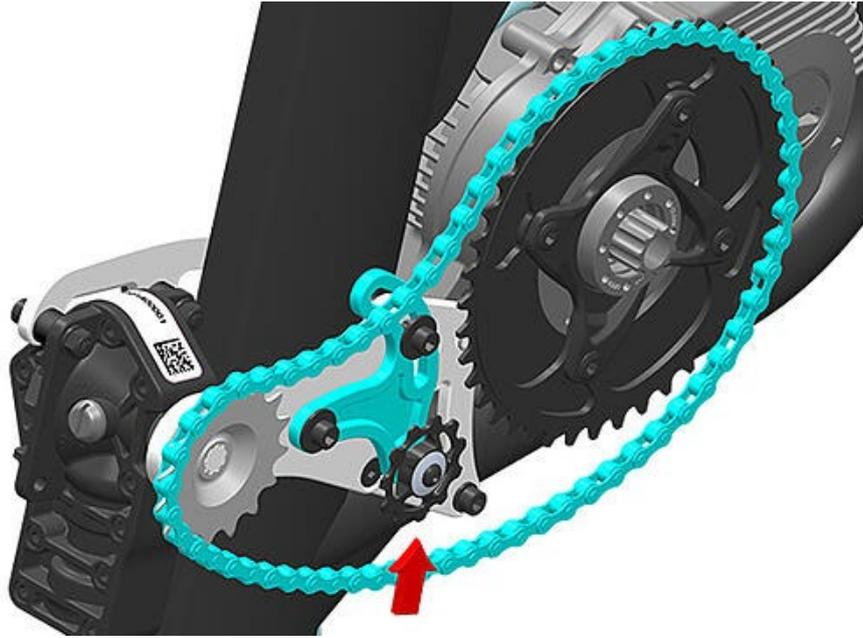
5.3 Apply light pressure (about 1kg of force) to the top of the Chain Tensioner Bracket and fasten the chain tension locking screw positioned in the slot at the same time.
