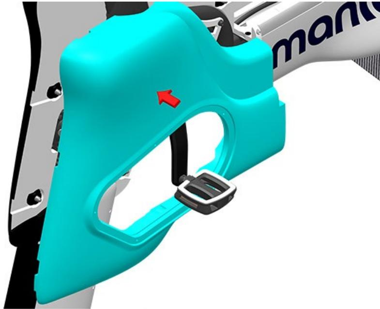
**INFORMATION:** If the RH Cranks is fitted, the Chain Guard must be removed before fitting the Rear RH Buoyancy to the bike.
