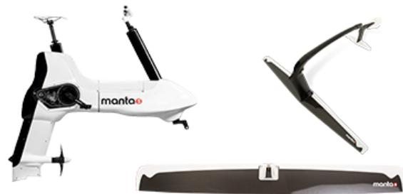
Before transporting the bike in the back of your car, make sure to remove the rear foil and front tiller assembly. Once these parts are removed we recommend the following transportation configuration based on the type of car your using:
