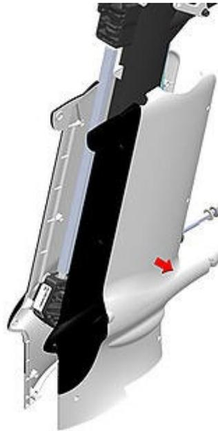
**INFORMATION :** Removal of the Strut Cowl provides access to the Top and Bottom Gearbox, Vertical Drive Shaft, Bayonet (Frame to Foil attachment) and Propeller Drive Shaft Assembly.
