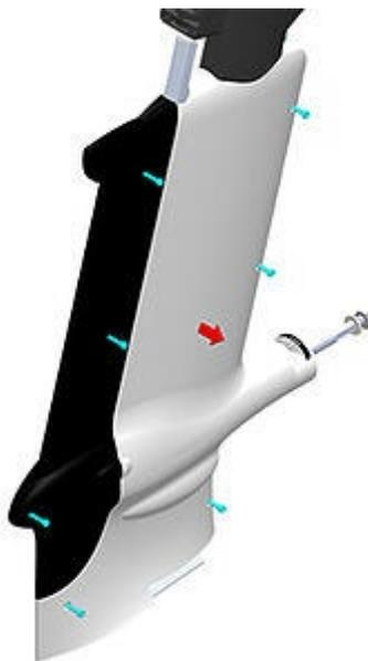
3.2 Unlock the Strut Collar by rotating anti-clockwise through 70 degrees. Remove the Collar by sliding it forward over the Propeller Drive Shaft.
