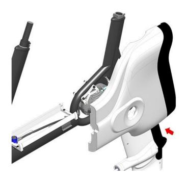
1.2 Position and hold Right-Hand Rear Buoyancy Module.
