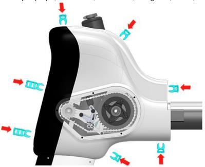
**INFORMATION:** Corresponding with the black and white colours of the Rear Buoyancy, four short white clips are fitted around the front, two long black clips at the rear and one short black clip is fitted on top behind the Seat Tube Clamp.
