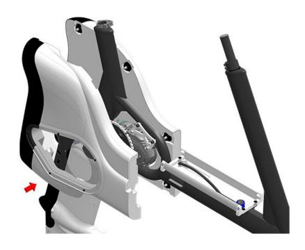
**INFORMATION:** As soon as the two Rear Buoyancy halves are in position, insert one of the Buoyancy Clips (white clip in front of the Seat Tube is a good option) so that the assembly is self-supported.
