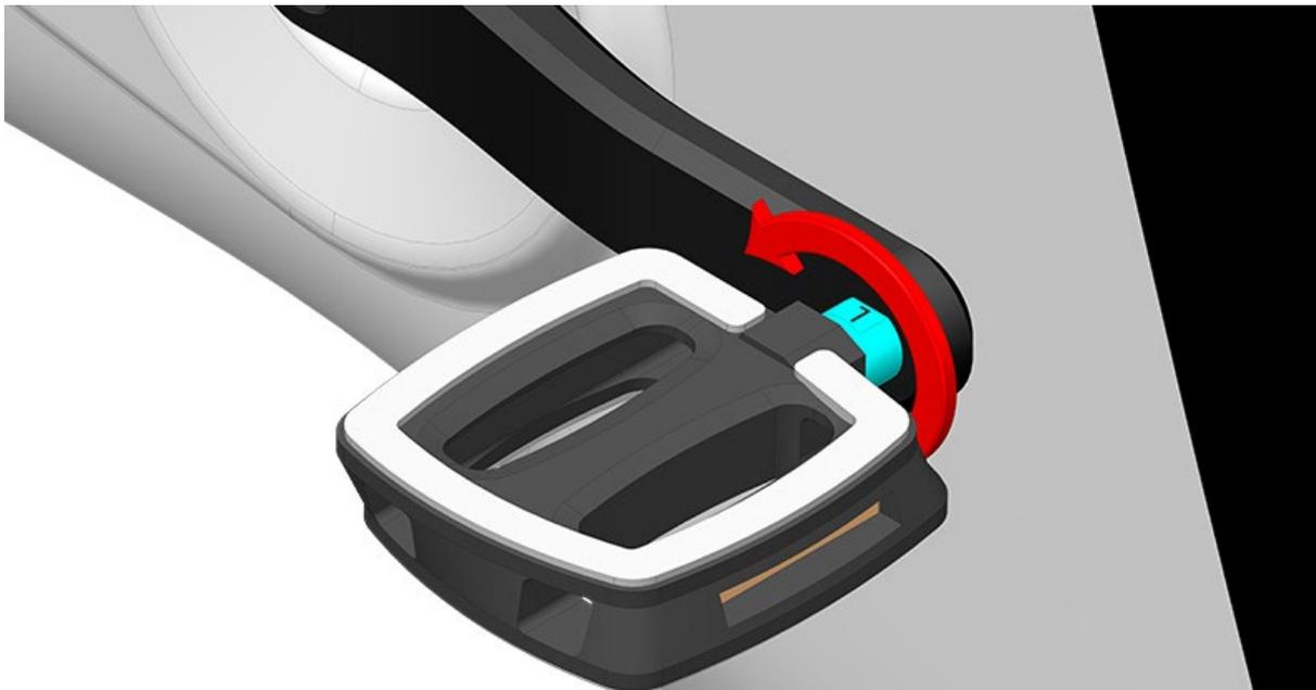
**INFORMATION:** As with standard bicycle parts, the Left-Hand Pedal has a left-hand thread and the Right-Hand Bike Pedal has a right-hand thread. It is strongly recommended that a pedal wrench with a minimum of lever length of 200 mm is used.
