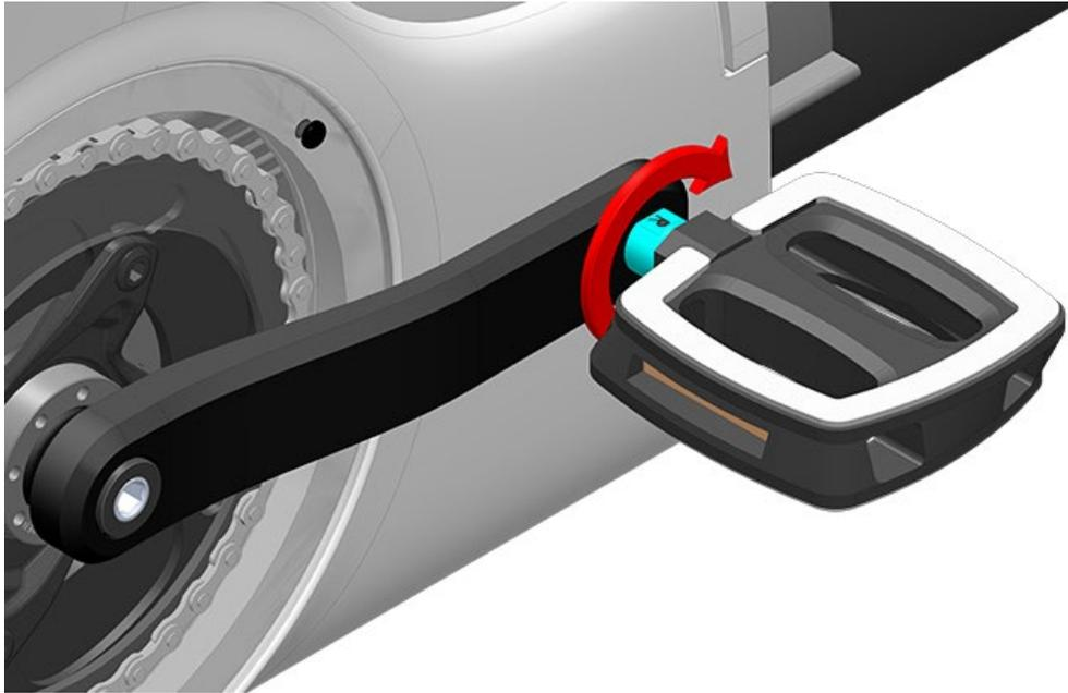
**INFORMATION:** The Right-Hand Pedal and Right-Hand Crank Arm have matching right-hand threads. If the Crank Arm does not accept the Right-Hand Pedal, check the markings on Pedal Shaft and Crank Arm.
