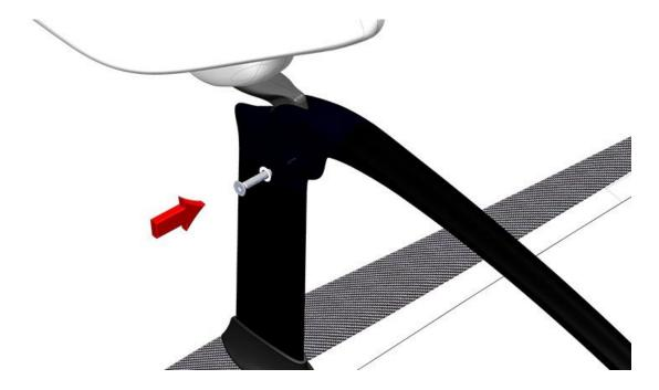
1.4 Fasten the screw. Do not over tighten; torque to 4 Nm with a 5mm Hex Key.
