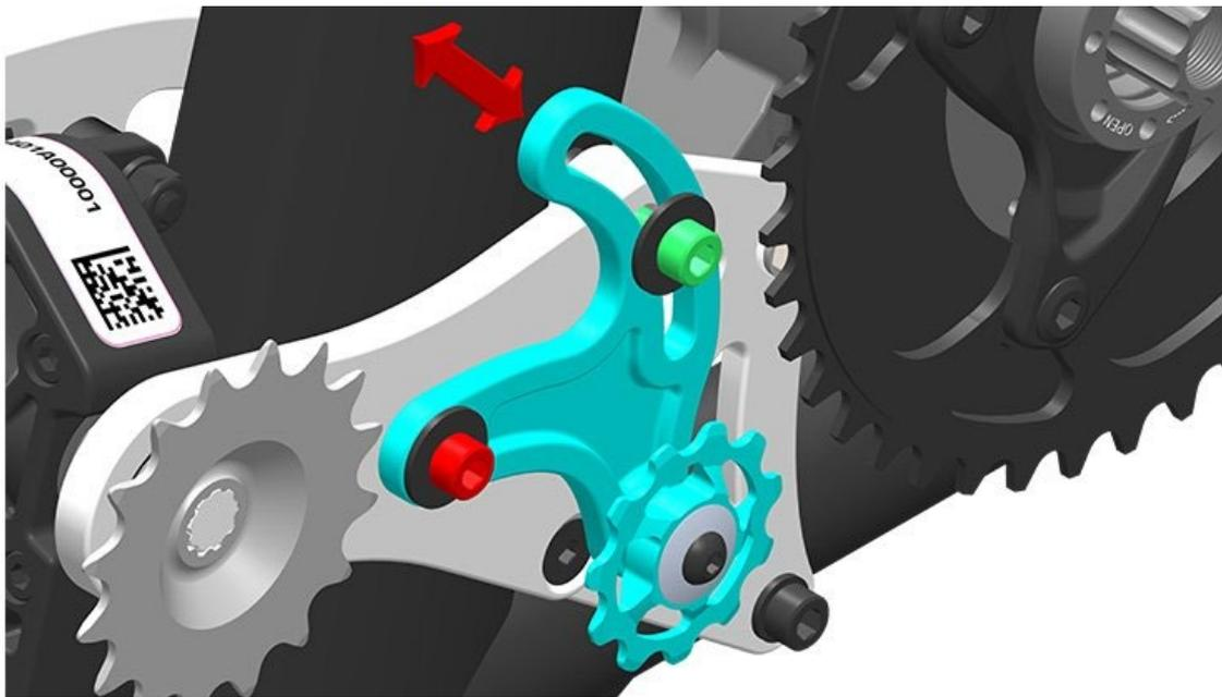
**INFORMATION:** The Chain Tensioner Assembly with Pulley (Jockey wheel) pivots around one screw serving as an axis (highlighted in red). The adjustment range is constrained by the slot and once adjusted the assembly is secured by firstly fastening the chain tension locking screw (highlighted in green) and finally the pivot screw. Do not use Loctite thread locker to the threads of the Chain Tensioner screws but use a lubricant like Tef-Gel (or equivalent) lubricant.
