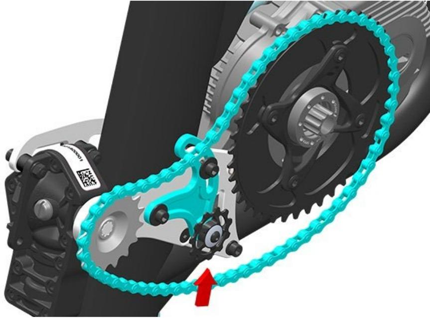
1.3 Apply light pressure (about 1kg of force) to the top of the Chain Tensioner Bracket and fasten the chain tension locking screw positioned in the slot at the same time.
